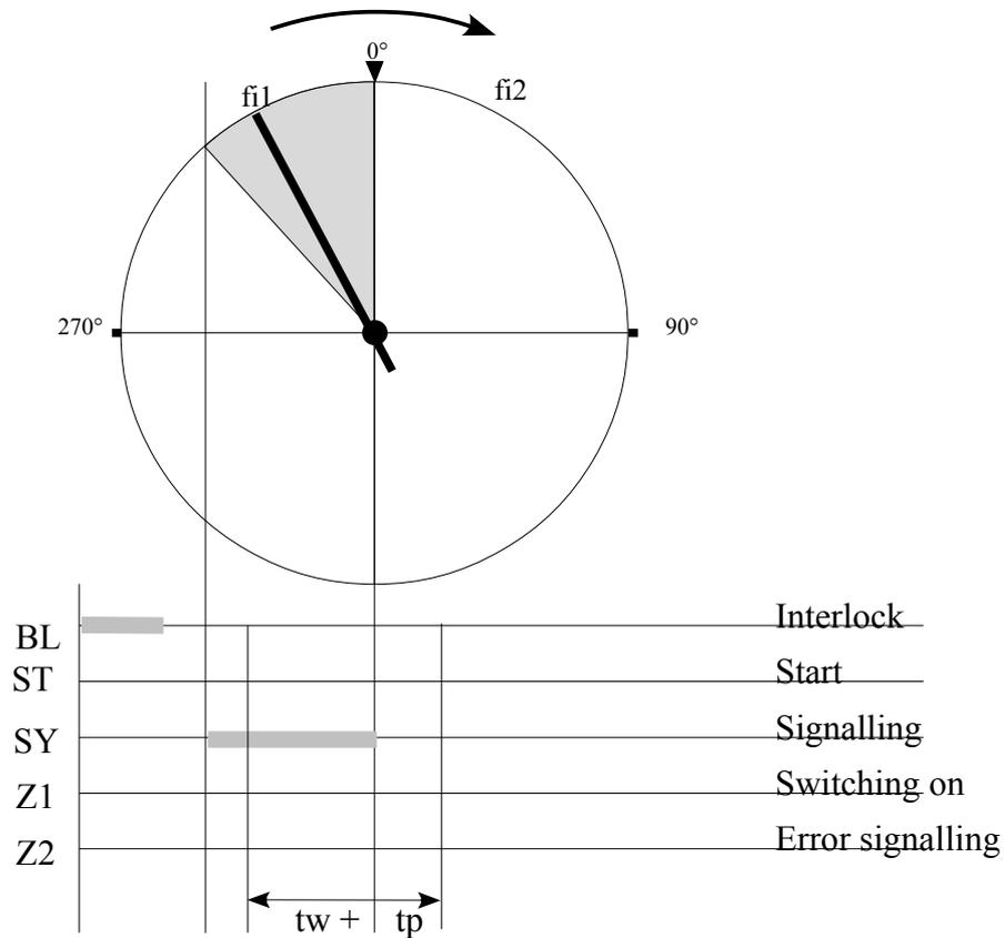
Fig.7. No switching pulse caused by the lack of a ST signal (start)
