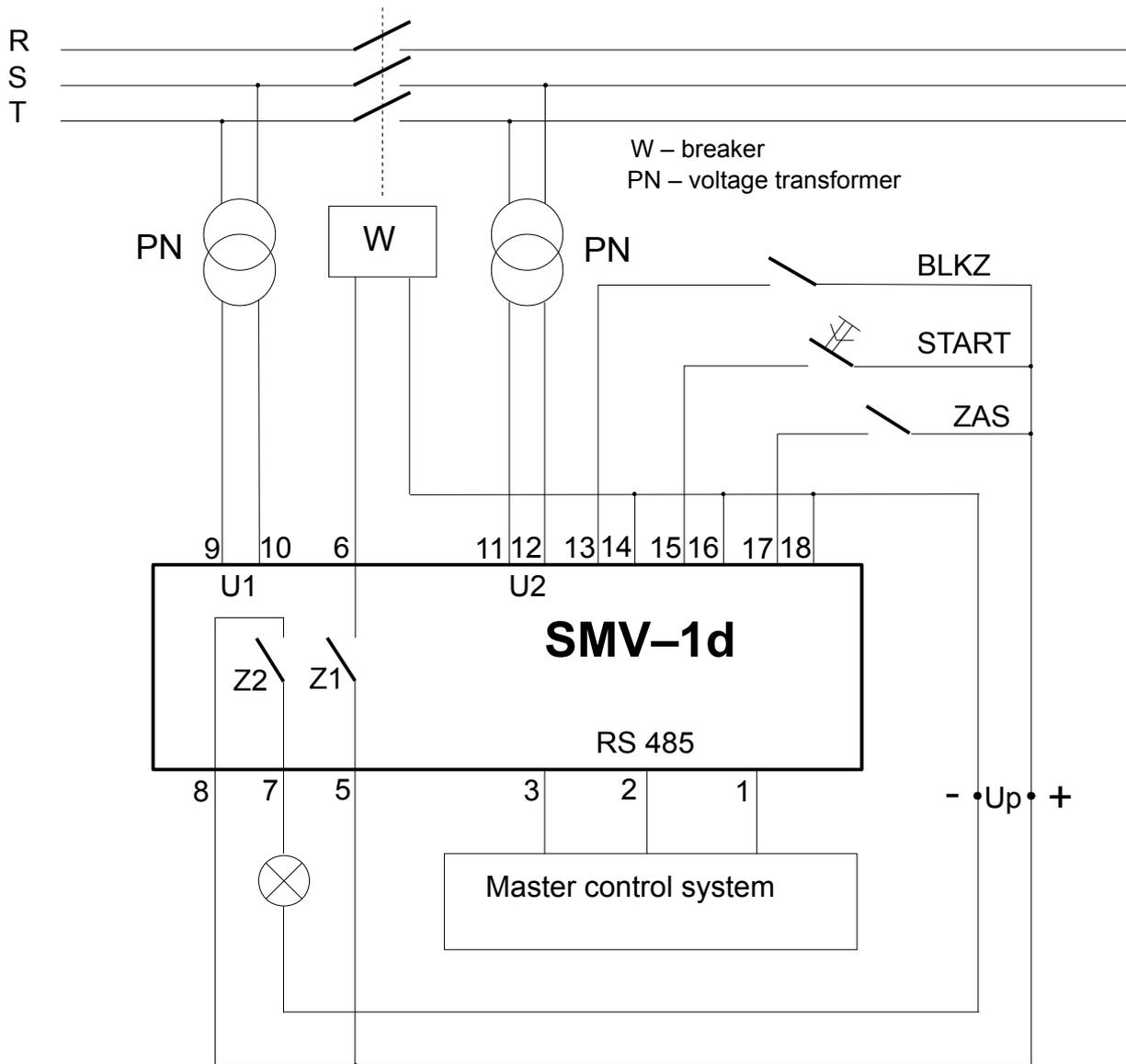
Fig. 3. Simplified diagram showing, how to connect the SMV-1d device to external circuits
