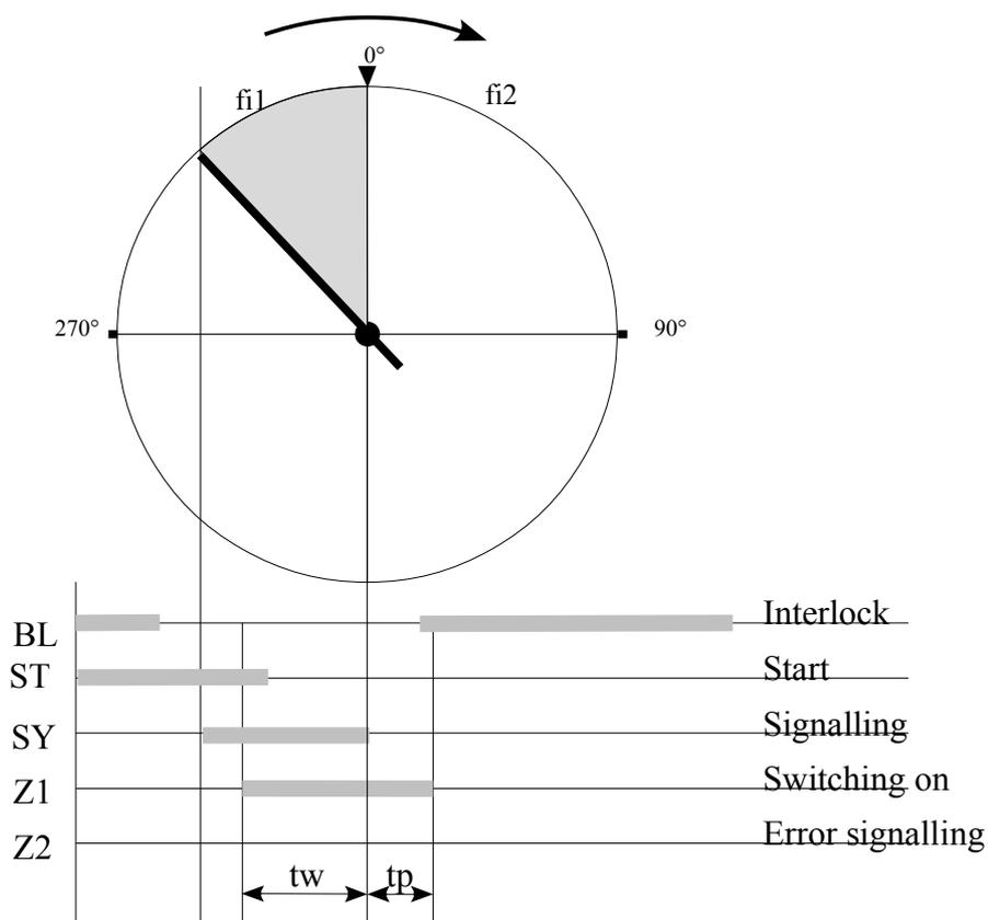
Fig. 8. Diagram of signals with the correct connection
